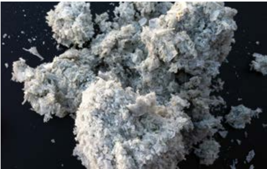
Wet fines derived from RPET bottles. Material clumps due to slight presence of label glue.
