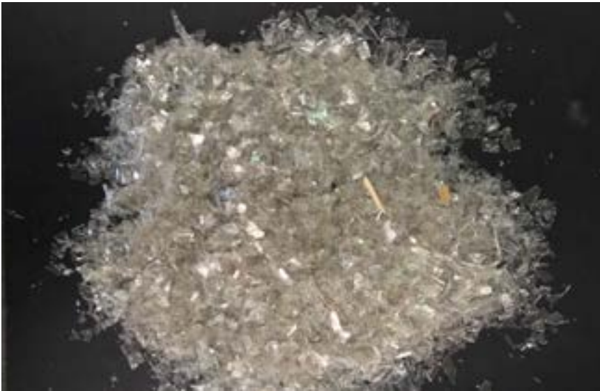
PET sheet regrind from floor space around grinders. May contain wood, paper, and/or dust contamination.
