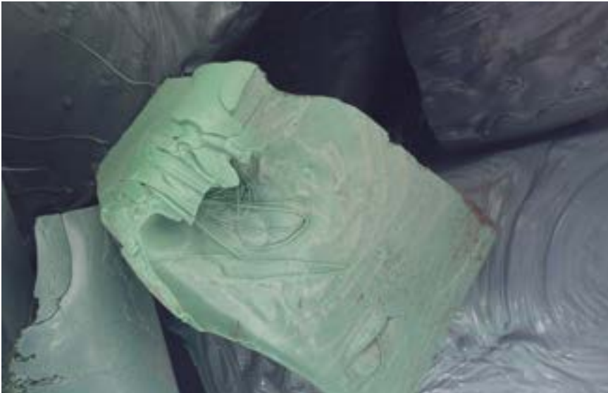
Green and Black RPET purge from Pelletizer and Sheetline. May contain backflush.
