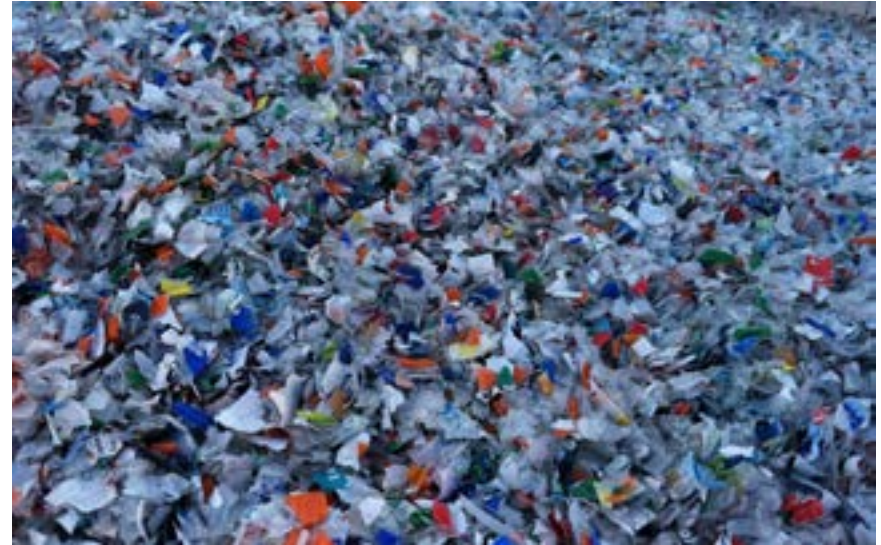
PP cap and label from RPET bottles. Wet, usually ships at approximately 10% moisture content.
