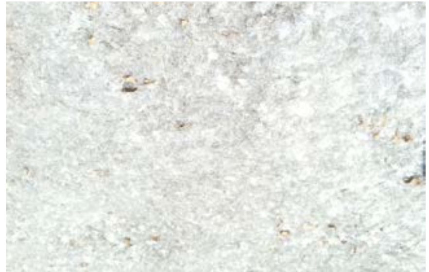
Clear regrind from RPET rollstock and thermoforms. Contains silicone coating. Contaminated with bits of tape and paper from roll core.
