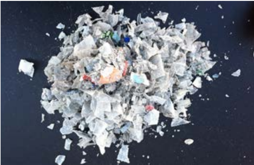
Wet Fines/Flake derived from RPET bottles. Contains contamination from metal, cap and label.
